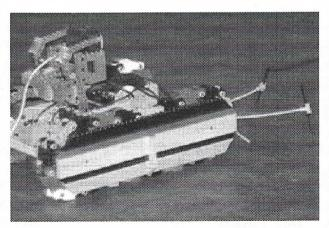
Above we have a wire controlled robot, Sir Cam-a-bot. This was built by Bazooka. He used Lego Technics to build this, and controlled the robot with a wire controller. The wire controller means no hassle with interference, but you need a lot of wire, and then of course one 'snip' and control is gone. He built this over a number of nights, coming up with this unique design.
