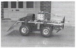
Starting with a simple remote control 4x4, we removed the body, then we attached Meccano, and built a large shield for the front. On the rear we attached rods of metal, which have a spearing effect. To finish this one we went a bit further, and attached some Meccano to the chassis; to this we attached a flail, again using Meccano.
