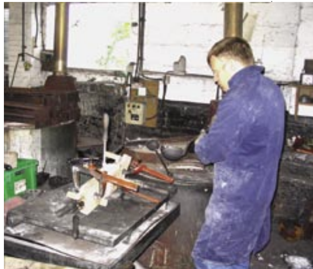
2. Pouring metal from a ladle into the clamped die. The top of the melting 'pot' can be seen at the rear.
