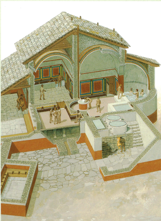
Above: A glass flask, found at Corbridge, which would have held the oil used in bath houses; oil was used instead of soap Below: A cutaway reconstruction of the bath house at Vindolanda, showing the methods of heating the floors and the walls. A replica of Chesters bath house can be seen at Wallsend (see page 33)
