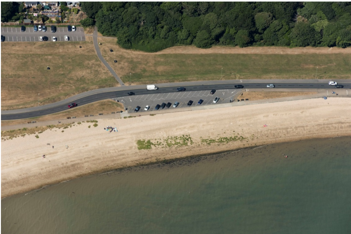
Figure 46. Looking north towards the concrete apron (under car park) and concrete matting (under sea weed on the foreshore) at embarkation hard G1. The circular patch in the centre left of the image is from a storage tank associated with the amphibious tank facility. (33560_018 26/06/2018 ©Historic England Archive).
