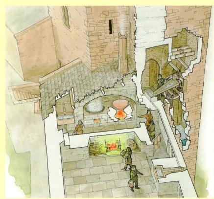
— a total of perhaps 600 people every day. As originally planned, but never completed, it was intended that supplies would be shipped into a dock just outside the Well Tower, and there unloaded directly into the tower's large basement store room. The gateway here was strongly defended by two pairs of doors and a portcullis. A stair wide enough for two porters to pass led up to the lower ward, where the granaries and larders were probably located.
