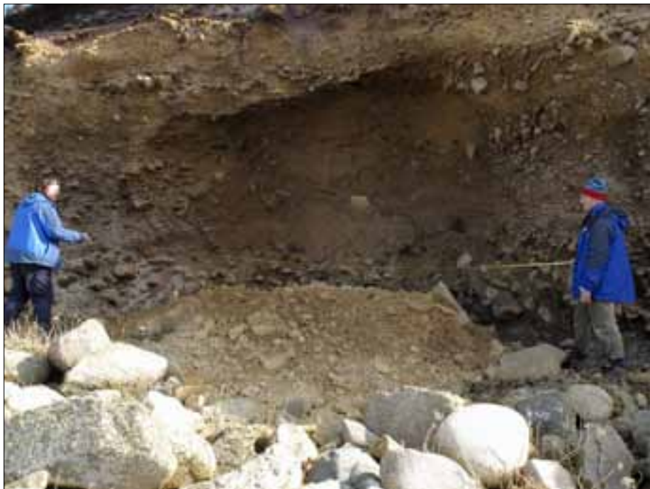
PI 35: Allan Brodie and the author measuring erosion undercutting the cliffs on the Garrison. (EH NMR DPI16017: 9 March 2010)
