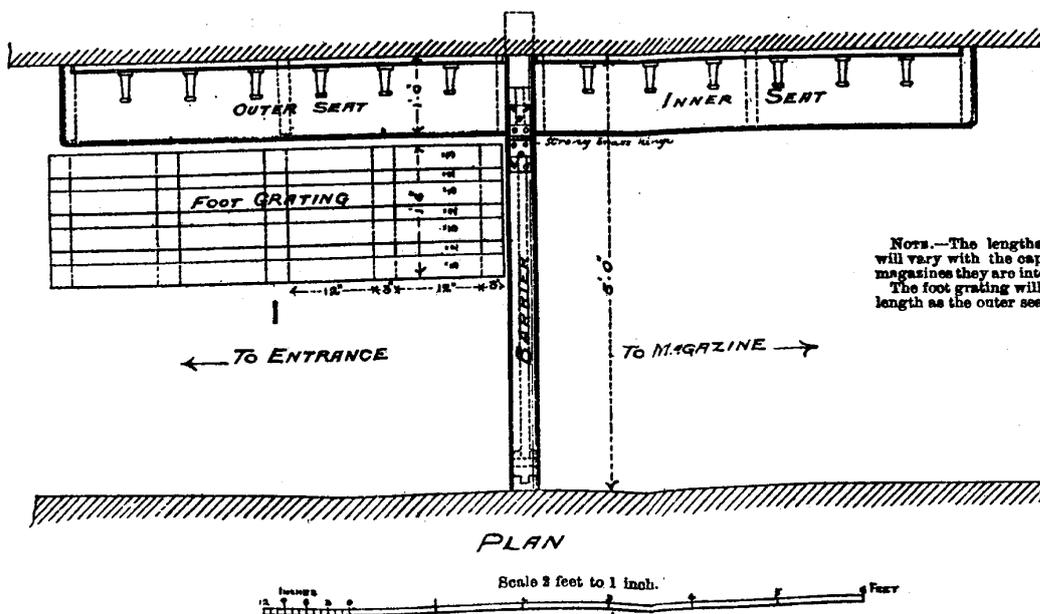
NOTE.—The lengths of the seats will vary with the capacities of the magazines they are intended to serve. The foot grating will be the same length as the outer seat.
